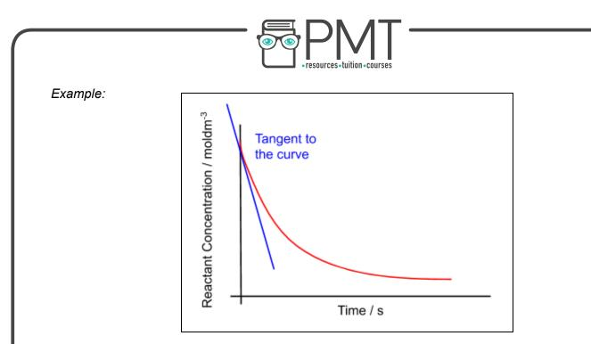
This method can then be repeated at varying concentrations to get a set of data for concentration and rate of reaction. This helps to identify the **relationship** between reactant concentration and rate.
