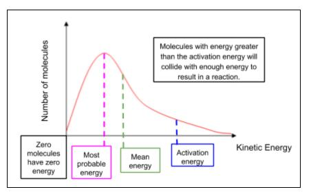
The total **area under the curve** represents the **total number of molecules** in the sample, therefore it must remain constant.
